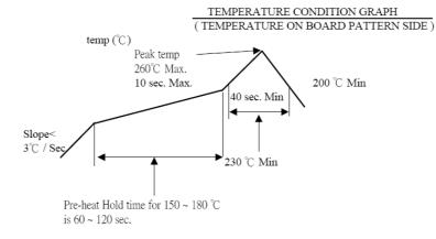
Notes: Thickness of the cream solder shall be maintained 0.12mm Min.
